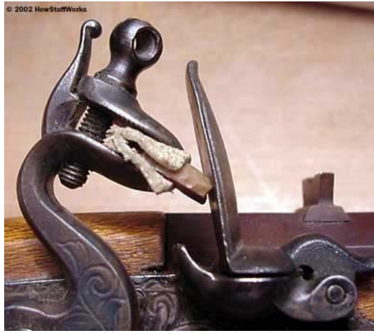
The frizzen at the flint's point of impact
